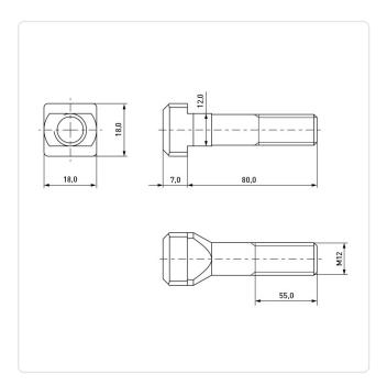
DIN/ISO: **DIN787** Finish: Plain Head Height [mm]:
