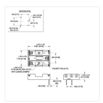
Battery Type: AAA-Micro Flammability Class: UL94-HB Length [mm]: 52.5
