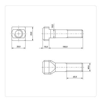
DIN/ISO: **DIN787** Plain Finish: Head Height [mm]:
