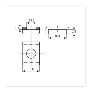
Finish: Plain For Thread Size: M5 Height [mm]: 1.2 Inner Diameter [mm]: 5.5
