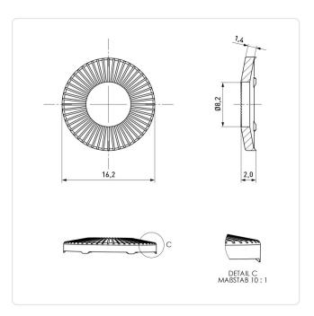
Finish: Plain For Thread Size: M8 Height [mm]: 1.4 Inner Diameter [mm]: 8.2
