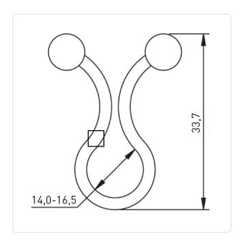
Bundle Diameter [mm]: 10,0-25,0 Color: Natural Flammability Class: UL94-V2 Material: PA 6.6 Material Group: **Plastic**
