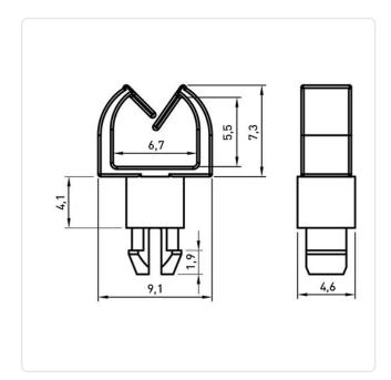
Bundle Diameter [mm]: 3,0-6,5 Color: Natural Height [mm]: 4.1 Material: PA 6.6 Material Group: **Plastic** Mounting Hole [mm]: 3.8 Panel Thickness [mm]: 1,6 mm 9.1 Width [mm]: Weight: 0.23g
