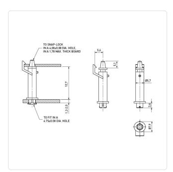
Color: Natural Flammability Class: UL94-V2 12.7 Length [mm]: PA 6.6 Material: Material Group: **Plastic** PCB Hole Ø [mm]: PCB Thickness [mm]: 1,8 Panel Hole Ø [mm]: 4.8 Panel Thickness [mm]: 1,2-2,0
