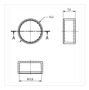
Color: Black Head Height [mm]: 7 Inner Diameter [mm]: 12.8 Material: PA 6.0 Material Group: **Plastic**
