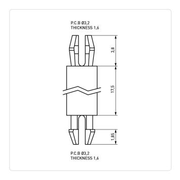
Color: Natural Flammability Class: UL94-V2 Length [mm]: 17.5 PA 6.6 Material: Material Group: **Plastic** PCB Hole Ø [mm]: 3.2 PCB Thickness [mm]: 1,6 Panel Hole Ø [mm]: 3.2 Panel Thickness [mm]: 1,6 Weight: 0.36g
