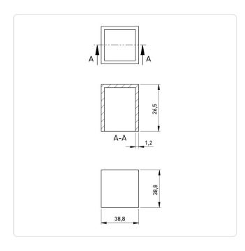
Color: Black Flammability Class: UL94-V2 Height [mm]: 26.5 38.8 Length [mm]: PA 6.6 Material:
