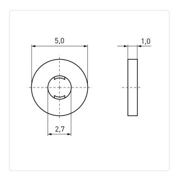
Color: Blue For Thread Size: M2.5 Height [mm]: Inner Diameter [mm]: 2.7
