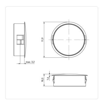
Color: Black Flammability Class: UL94-V2 Head Diameter [mm]: 11.9 Head Height [mm]: 1.6 PA 6.6 Material: Material Group: Plastic Snap-In Model: Mounting Hole [mm]: 9.5
