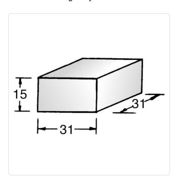
Height [mm]: 15 Length [mm]: 31 Material: Steel Material Group: Steel Width [mm]: 31 Weight: 15g Conformities:
