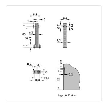
Color: Gray Dist. Mounting Holes [mm]: 12.7 Flammability Class: UL94-V0 60
