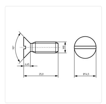
Color: Natural Drive Type: Slotted Head Diameter [mm]: 14.5 Head Height [mm]: 6.65
