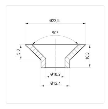
Color: Natural Flammability Class: UL94-V2 Inner Diameter [mm]: 10.2 Lug Diameter [mm]: 12.4 Material: PA 6.0
