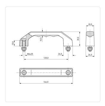
Color: Black Dist. Mounting Holes [mm]: 120 Height [mm]: 39 Material: PA 6.0 Material Group: Plastic
