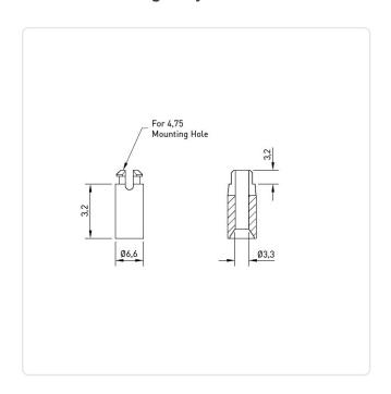
Color: Natural Flammability Class: UL94-V2 For Thread Size: М3 Inner Diameter [mm]: 3.3 Length [mm]: 3.2 Material: PA 6.6 Material Group: Plastic Mounting Hole [mm]: 4.75 Outer Diameter [mm]: 6.6
