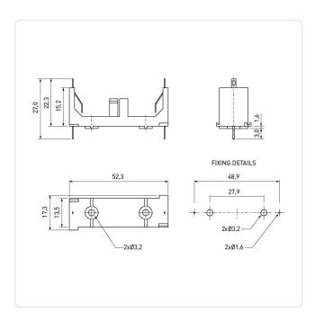
Battery Type: AAA-Micro Flammability Class: UL94-V0
