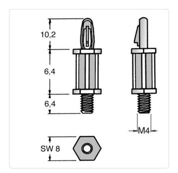
Color: Natural Flammability Class: UL94-V0 Length [mm]: 6.4 Material: PA 6.6 Material Group: **Plastic** PCB Hole Ø [mm]: PCB Thickness [mm]: 1,6 Thread Size: M4 Weight: 0.44g
