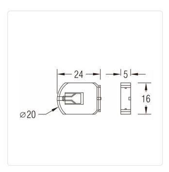
Battery Type: Cell Dia. 20mm
