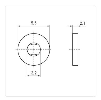
Color: Gray For Thread Size: М3 Height [mm]: 2.1 Inner Diameter [mm]: 3.2 Material: PA 6.6 Material Group: Plastic Outer Diameter [mm]: 5.5 Weight: 0.03g
