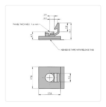
Color: Natural Flammability Class: UL94-V2 Length [mm]: 6.5 Material: PA 6.6 Material Group: Plastic PCB Thickness [mm]: 1,6 1.18g
