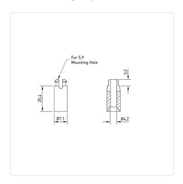
Color: Natural Flammability Class: UL94-V2 For Thread Size: M4 Inner Diameter [mm]: 4.2 Length [mm]: 25.4 Material: PA 6.6 Material Group: Plastic Mounting Hole [mm]: 5.9 Outer Diameter [mm]: 7.1 Weight: 0.78g
