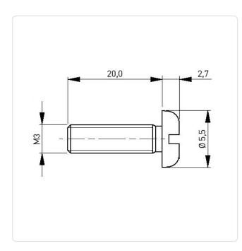
Color: Natural Drive Type: Slotted Head Diameter [mm]: 5.5 Head Height [mm]: 2.7
