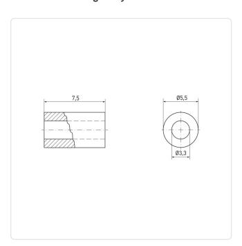
Finish: Plain For Thread Size: М3 Inner Diameter [mm]: 3.3 Length [mm]: 7.5
