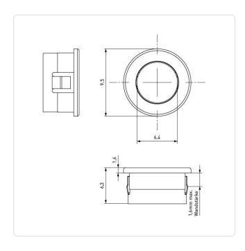
Color: Black Inner Diameter [mm]: 6.4 Material: PA 6.6 Material Group: Plastic Max. Panel Thickness [mm]: 1.6 Mounting Hole [mm]: 8 Outer Diameter [mm]: 9.5 Weight: 0.12g
