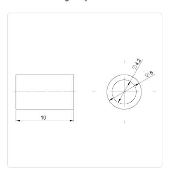
Finish: Plain For Thread Size: M4 Inner Diameter [mm]: 4.2 Length [mm]: 10
