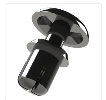
Color: Black UL94-V2 Flammability Class: Head Diameter [mm]: 6.4 Head Height [mm]: 1.6 Length [mm]: 5.5 Material: PA 6.6 Material Group: Plastic Model: removable Mounting Hole Range [mm]: Ø 3.6-3.7
