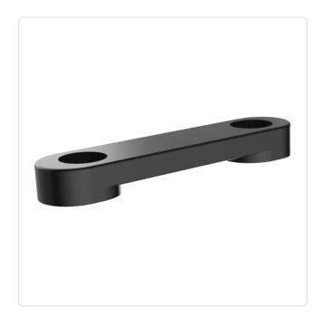
Bundle Diameter [mm]: 9 Color: Black Distance Middle/Middle [mm]: 16 Length [mm]: 23 PA 6.6 Material: Material Group: Plastic Mounting Hole [mm]: 3.2 Thickness [mm]: 3 Width [mm]: 7 Weight: 0.38g
