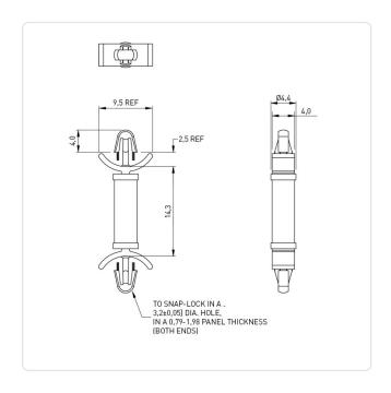
Color: Natural Flammability Class: UL94-V2 14.3 Length [mm]: PA 6.6 Material: Material Group: **Plastic** PCB Hole Ø [mm]: 3.2 PCB Thickness [mm]: 0,8-2,0 Panel Hole Ø [mm]: 3.2 Panel Thickness [mm]: 0,8-2,0 Weight: 0.32g
