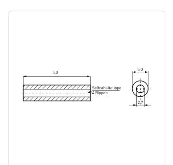
Color: Black Flammability Class: UL94-V2 For Thread Size: M2.5 Inner Diameter [mm]: 2.7 Length [mm]: 5 Material: PA 6.6 Material Group: **Plastic**
