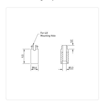
Color: Natural Flammability Class: UL94-V2 For Thread Size: M3 Inner Diameter [mm]: 3.3 Length [mm]: 9.5 Material: PA 6.6 Material Group: Plastic Mounting Hole [mm]: 4.8 Outer Diameter [mm]: 6.6
