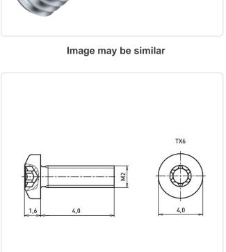
Torx T6 Actuator Size: DIN/ISO: ISO14583 Drive Type: **TORX**
