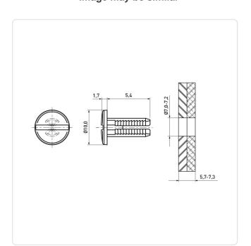
Color: Black Head Diameter [mm]: 10 Material: PA 6.6 Material Group: Plastic Mounting Hole [mm]: 7.1
