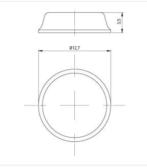
Bumper Design:Round, TaperedColor:WhiteDiameter [mm]:12.7Height [mm]:3.5Material:PUR - PolyurethaneMaterial Group:PlasticWeight:0.63gConformities:ReachReachCOMPLIANTCOMPLIANTCOMPLIANT
