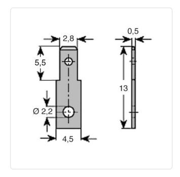
Bending Angle [°]: Plain Finish: Length [mm]: 13 Material: Brass Material Group: Brass Mounting Hole [mm]: 2.2 Plug-In Length [mm]: 5.5 Size [mm]: 2.8x0.5 Tabs: Weight: 0.17g
