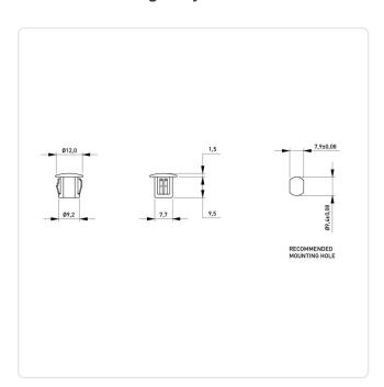
Color: Black PA 6.6 Material: Plastic Material Group: Model: Snap-In Mounting Hole [mm]: 9.4 Outer Diameter [mm]: 12 Weight: 0.39g
