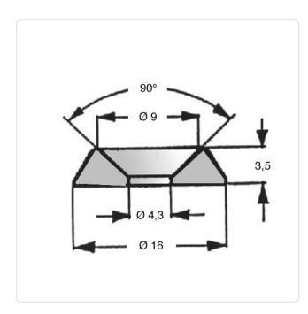
Color: Black For Thread Size: M4 Height [mm]: 3.5 Inner Diameter [mm]: 4.3 Material: PA 6.0 Material Group: Plastic Outer Diameter [mm]: 16 Weight: 0.49g
