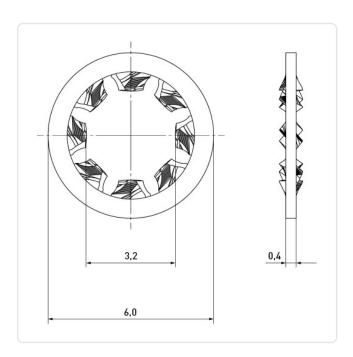
DIN/ISO: **DIN6798I** Finish: Plain For Thread Size: М3 0.4 Height [mm]: Inner Diameter [mm]: 3.2
