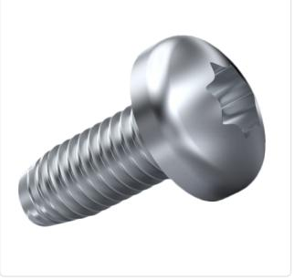
Actuator Size: Torx T8 DIN/ISO: DIN7500-C Drive Type: **TORX** Plain Finish: Head Diameter [mm]: 5 Head Height [mm]: 2.2
