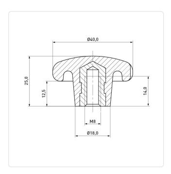
Color: Black Diameter [mm]: 40 Height [mm]: Material: Plastic Material Group: Plastic Thread Size: M8 Weight: 20.76g
