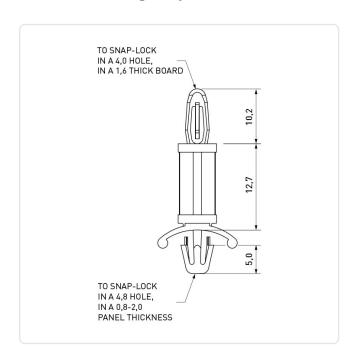
Color: Natural Flammability Class: UL94-V2 Length [mm]: 12.7 PA 6.6 Material: Material Group: **Plastic** PCB Hole Ø [mm]: PCB Thickness [mm]: 1,6 Panel Hole Ø [mm]: 4.8 Panel Thickness [mm]: 0,8-2,0
