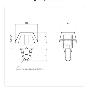
Color: Natural Head Diameter [mm]: 12.3 Material: PA 6.6 Material Group: Plastic Mounting Hole [mm]: 4.8
