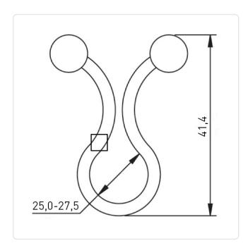
Bundle Diameter [mm]: 20,0-25,0 Color: Natural Flammability Class: UL94-V2 Material: PA 6.6 Material Group: **Plastic** Weight: 0.99g
