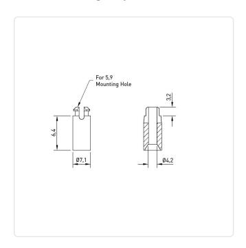
Color: Natural Flammability Class: UL94-V2 For Thread Size: M4 Inner Diameter [mm]: 4.2 Length [mm]: 6.4 Material: PA 6.6 Material Group: Plastic Mounting Hole [mm]: 5.9 Outer Diameter [mm]: 7.1
