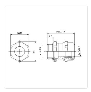
AF / OD [mm]: 19 Black Color: Material: PA 6.0 Material Group: Plastic Mounting Hole [mm]: 16.5 Panel Thickness Range [mm]: 4.5-10.0 Protection Code: **IP68** Thread Size: M16 Weight: 6.12g
