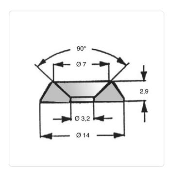
Color: Black For Thread Size: МЗ Height [mm]: 2.9 Inner Diameter [mm]: 3.2 Material: PA 6.0 Material Group: Plastic Outer Diameter [mm]: 14 Weight: 0.34g
