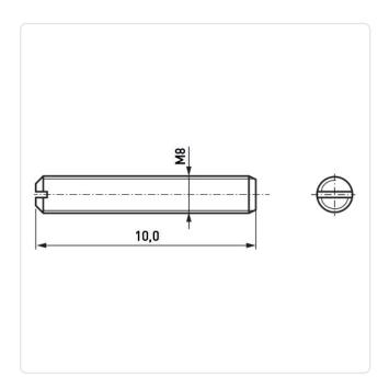
Color: Natural DIN/ISO: ISO4766 Drive Type: Slotted Flammability Class: UL94-V2 Length [mm]: 10 Material: PA 6.6 Material Group: Plastic Point Type: Flat Point Thread Size: M8 0.45g
